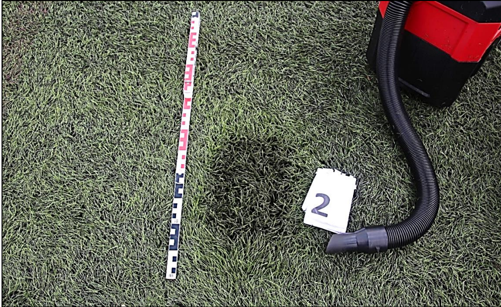
Figure 3: Vacuuming the infill material
