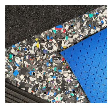
The quality of shockpads continues to improve, meaning those on the market today should be able to function adequately under at least two synthetic turf carpets (so typically 15 to 20 years). This has not always been the case, and the shockpads laid under turfs in the past might need replacing when the initial turf is replaced. At some point, however, all shockpads will need to be replaced, and currently the following options are available:
