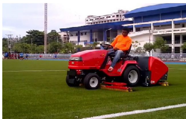
Figure 3 - brushing of a synthetic turf field with specialist equipment that captures any debris or detritus found on the field.
