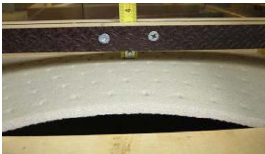
Figure C.3 – example of shockpad bowing (concave)
